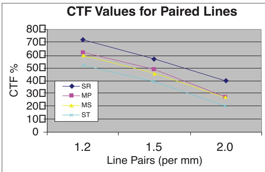
Figure 5. Each screen is able to resolve line pairs to different degrees as measured quantitatively by the CTF values. SR screens give the best resolution to the line pairs.
