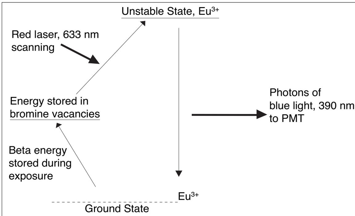
Figure 1. Schematic representation of the storage phosphor process.
